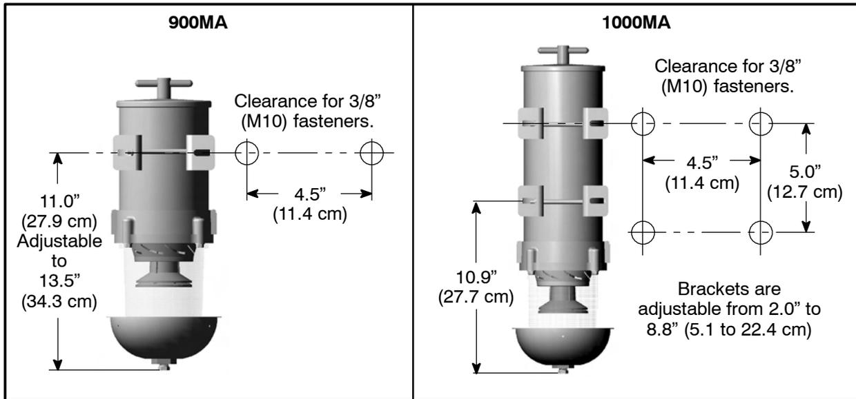
**Note** - mount the filter assembly as close to vertical (**V**) as possible. Do not exceed 10° from vertical or the assembly may not function properly.
